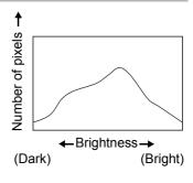
image. In general, when the exposure meter setting for your image is well-balanced, the graph peaks tend to appear in the middle. On the contrary, when the exposure meter gets imbalanced tending dark and bright without showing a neutral brightness, the peaks appear not in the middle but on both sides.
